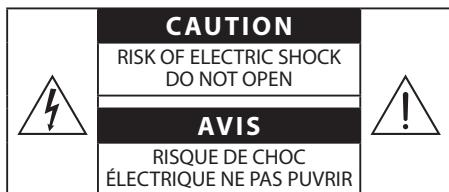
The lightning flash with arrowhead symbol, within an equilateral triangle, is intended to alert the user to the presence of uninsulated "dangerous voltage" within the product's enclosure that may be of sufficient magnitude as to constitute a risk of electric shock to persons.
